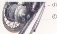
Fig. 34 ① Rr. brake panel ② Reference mark ③ Indicator ④ Rr. brake arm
